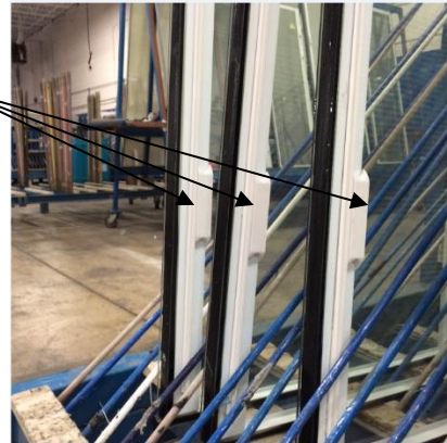
Operator Down Position
