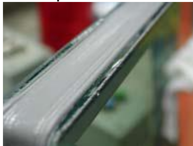
Acceptable Squeeze-out ≤ 1/16"
